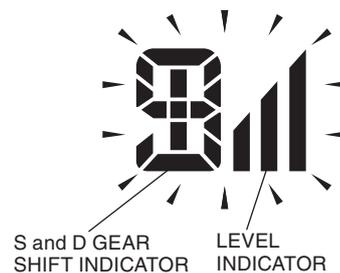
4. S gear shift indicator, level indicator and D gear shift indicator blink alternately 5 seconds after deregistration is completed.
